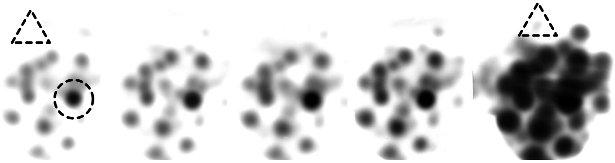
Figure 3: Time series of photographic paper, located at the end of the solenoid, exposed 30 s, 45 s, 1 min, 2 min and 5 min. The individual pictures have been taken during the course of a day. The image is remarkably stable in this time frame.
