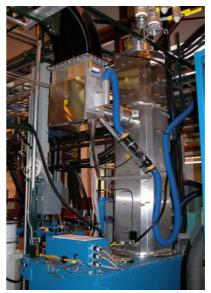
Figure 1: 402.5 MHz, 2.5 MW Klystron
