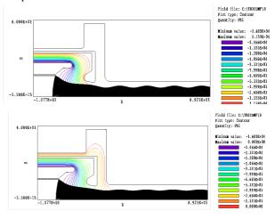
Figure 4: TRICOMP simulations in gun section. The potential at the cathode is -16kV; at the mod-anode is 0kV in top plot and -4kV in bottom plot.
