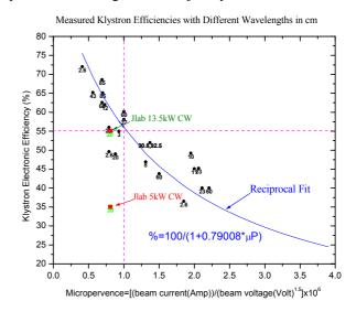
Figure 1: Klystron efficiency vs beam preveance.
