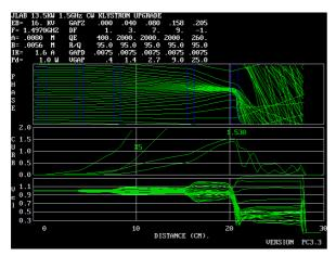
Figure 6: The JPNDIS simulation. Up to down: input parameters, Applegate plot, RF current verse z, velocity spread verse z.
