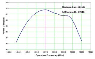
Figure 9: JPNDISK calculated gain and bandwidth.
