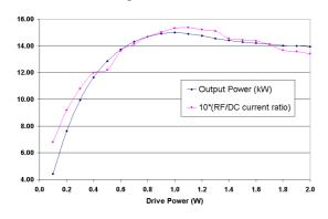
Figure 7: JPNDISK calculated output power verse input.
