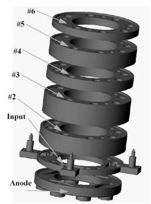
Figure 3. Exploded view of circuit assembly for first six cavities
