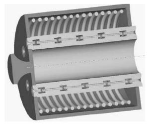
Figure 1. Solid model of multiple beam klystron with ring resonator cavities.
