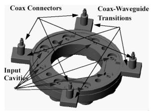
Figure 2. Input cavity assembly showing four coaxial inputs to waveguide transitions.
