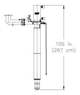
Figure 2: VKP-8291A Klystron Layout
