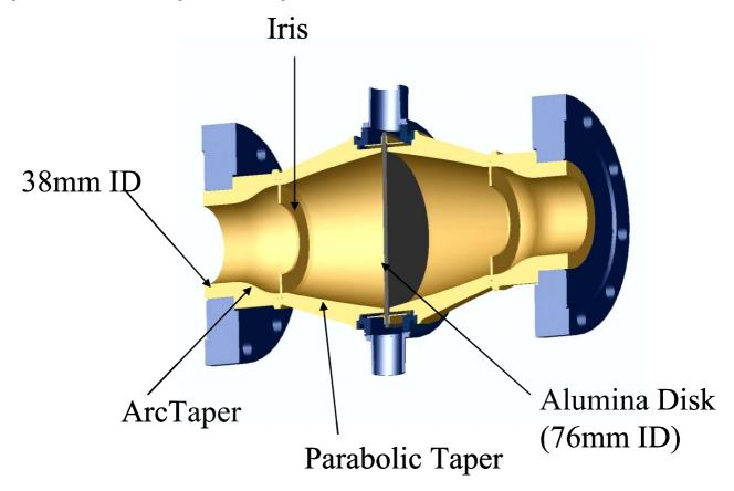
Figure 1. Cross section of high power X-Band window.
