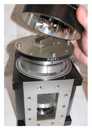
Figure 2: Switch head bearing and channel piece.
