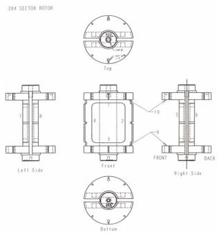
Figure 3: WR-284 rotor edges that are handworked.
