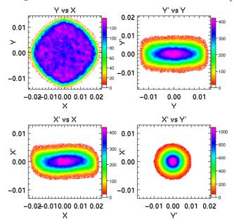
Figure 2: Configuration and phase space contour plots after 50 lattice periods for  $\sigma_0$ =60°, I=849 mA (fills 86% of radial aperture). Units of x and y are meters.
