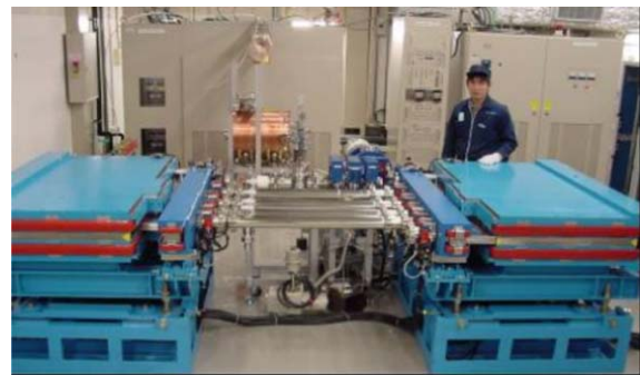
Figure 2: CW microtron and the RF power source.
