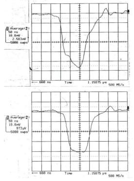
Figure 2: Magnetic field pulse at input (top) and output (bottom) of kicker magnet
