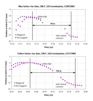
Figure 5: Beam based rise time measurements
