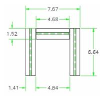
Figure 1: Kicker magnet core cross section (in cm)
