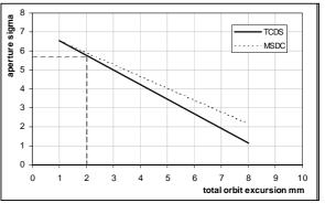
Figure 4. Aperture at 450 GeV for extracted beam as a function of the orbit in the nominal 15/15 MKD case.
