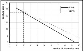
Figure 5. Aperture at 7 TeV for extracted beam as a function of the orbit in the nominal 15/15 MKD case.
