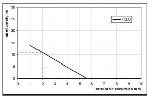
Figure 7. Aperture at 7 TeV for extracted beam as a function of the orbit in the 14/15 MKD case.
