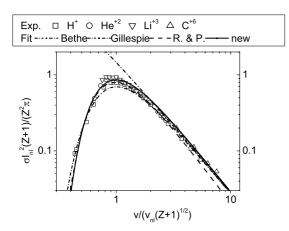
Figure 2: Ionization cross sections of hydrogen by fully stripped ions showing the scaled experimental data and the theoretical fits. BA denotes the Born approximation. Gillespie denotes Gillespie's fit. R.&P. symbolizes the fit proposed by Rost and Pattard [11]. "New" denotes the new fit given by Eq. (6).
