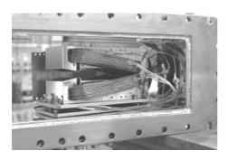
Figure 6: Picture of the massless septum magnet.
