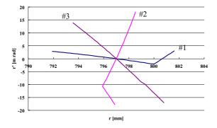
Figure 3: Shape of the beam in the phase space at the first masless septum magnet (#1), electrostatic septum (#2) and the second massless septum magnet (#3).
