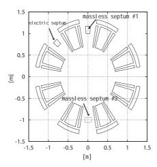
Figure 2: Configuration of the extraction system.
