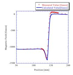
Figure 5: Magnetic flux density at the median plane plotted as a function of the horizontal position.
