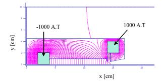
Figure 4: Upper half of the designed magnet. The calculated field lines are also presented in this figure.
