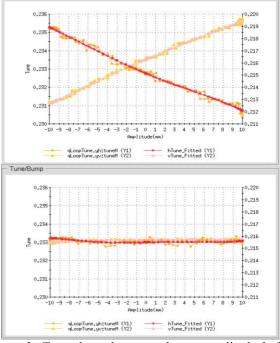
Figure 3. Tune dependence vs. bump amplitude before and after correction, IR8,  $\beta^*=2m$  optics.
