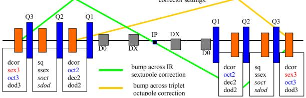
Figure 2. Schematics of a RHIC IR, with the IR correction system and IR bumps used for the correction
