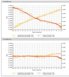
Figure 4. Tune dependence vs. bump amplitude before and after correction, IR8,  $\beta^*=1m$  optics.
