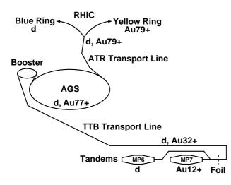
Figure 1: Acceleration of Deuterons and Gold for RHIC.
