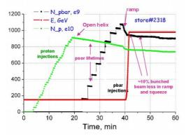
Figure 1: Beam intensity and loss during injection, ramping and squeeze
