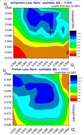
The tune scan shown in the figure above displayed the loss versus the working point. The proton and antiproton
