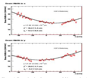
Figure 1 Example plot for one run of 20 runs showing luminous region size versus z and the fits to Equation 2. Typical correlation coefficients of the fits are about -0.8 for  $(\beta^*, \varepsilon)$ , 0.5 for  $(\beta^*, z_0)$ , and -0.6 for  $(\varepsilon, z_0)$
