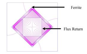
Figure 1: PANDIRA model of Panofsky quadrupole
