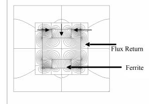
Figure 4: Halbach array skew quad arrows indicate direction of the field array
