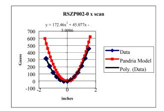
Figure 7: Hall probe scan of sextupole with Pandira model data
