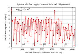
Figure 2: Radical beam separations at 138 interaction points in the ring.
