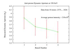
Figure 7: Measure Dynamic apeture at injection
