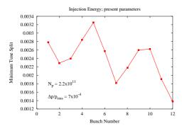
Figure 5: small amplitude beam-beam coupling at injection.
