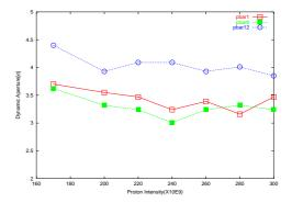
Figure 6: DA of  $\overline{p}$  vs. proton intensities at Cog2,  $10^5$  turns
