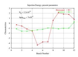
Figure 4: small amplitude beam-beam chromaticities at injection.
