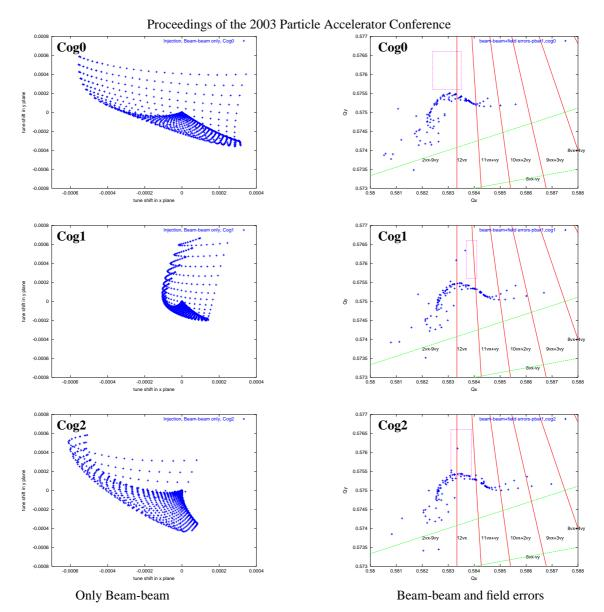
Figure 3: Footprint of  $\overline{P}$  bunch 1 at three cogging stages.
