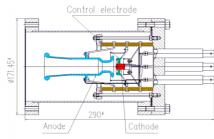
Figure 1: Electron gun structure
