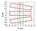
Figure 6: The path of the electron beam in the bends: designed (magenta) and measured (blue)
