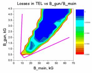
Figure 4: Electron losses in the path
