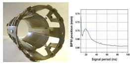
Figure 8: The prototype of new TEL BPM
