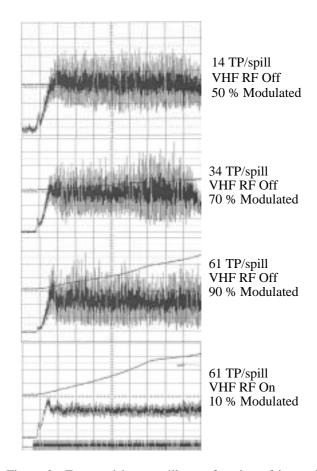
Figure 2: Extracted beam spill as a function of internal beam intensity with and without VHF on
