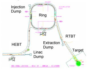
Figure 1: SNS Ring and Transport Line layout
