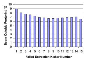
Figure 1: Fraction of beam outside the nominal target footprint for single extraction kicker failures. Number 15 shows the nominal value.
