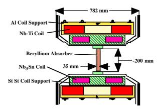
Figure 2. A Cross-section of the MICE Focusing Magnet with a Nb<sub>3</sub>Sn Insert Coil and a Beryllium Absorber
