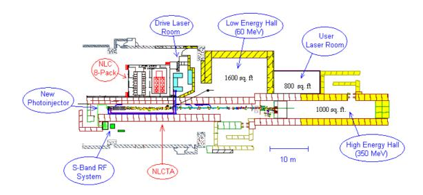
Figure 1. Conceptual layout of the ORION Facility at the NLCTA.
