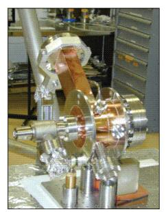
Figure 2. ORION rf gun after the final braze at SLAC.
