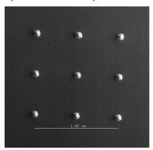
Figure 2: A 500  $\mu$ m period matrix etched on (100) Si[6].
