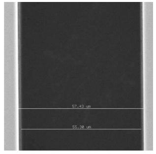
Figure 3: View of a 50  $\mu$ m slit etched along the [111] lines in a 500  $\mu$ m thick, (110) Si wafer. The wall height-to-thickness ratio is 500:1. Thinner slit widths are harder to view and thicker ones have worse resolution.
