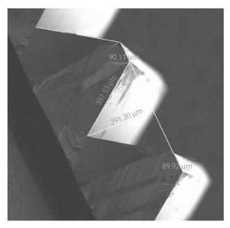
Figure 1: A 500  $\mu m$  period grating etched on (100) Si.
