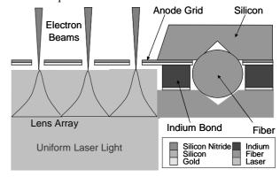
Figure 5: Schematic for a backlit, gated photocathode[5].
