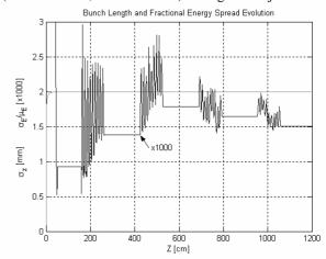
Figure 3. RMS bunch length and fraction energy spread (x1000) through the injector.
