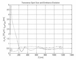
Figure 2. Transverse RMS beam sizes (solid curves, in units of  $10 \mu m$ ) and normalized (one-sigma) emittances (dashed curves, in units of nm) through the injector.
