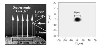
Fig. 2 Supersonic gas jet and laser focus position. Fig. 3 Image of the laser focal spot at the target.
