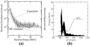
**Fig.4** The measured and calculated time-integrated (a) and spatial (b) energy distribution of electrons in the bunch for the laser power of 4TW.
