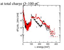
**Fig.6** Electron energy distribution in 2D PIC simulation;  $I=10^{20}$  W/cm<sup>2</sup>,  $\tau=20$  fs,  $\omega t=6000$  (b)  $\omega t=12000$  (b) at the plasma density  $N_e=10^{19}$  cm<sup>-3</sup>
