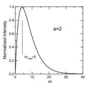
**Fig. 7** Typical spectrum of scattered x-rays [2]. The maximum frequency is  $\omega \sim m\omega_0 8 \gamma_0^2 / (1+a_0^2)$  with  $\gamma_0$  the energy of accelerated electrons.
