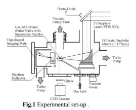
was placed inside the vacuum chamber. The pulse valve was driven for 5 ms a shot at a repetition rate of 0.2 Hz. The stagnation pressure of the valve is varied from 5 to 20 atm. With these pressures the density at the exit of the nozzle ranged from  $7 \times 10^{18}$  to  $3 \times 10^{19}$  cm<sup>-3</sup>.
