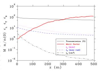
Figure 3: Performance of RFOFO Ring. Transmission, normalized transverse emittance, normalized longitudinal emittance, normalized 6-dimensional emittance, and the merit factor M, as a function of distance.
