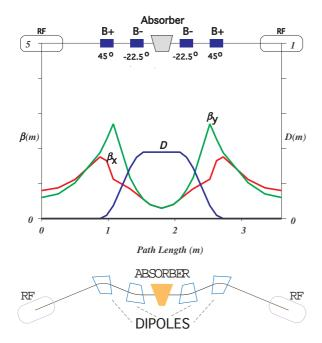
Figure 5: A dipole-only, 8-cell ring lattice including reverse bends. The pole-face angles and the reverse bending give 6D cooling as well as zero dispersion in the rf drift spaces.
