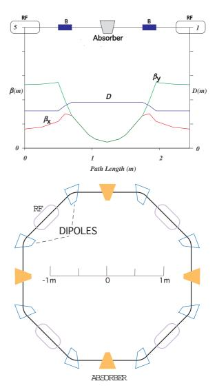
Figure 3: A dipole-only 4-cell ring lattice. The required focusing is accomplished by adjusting the dipole entrance and exit pole-face angles.
