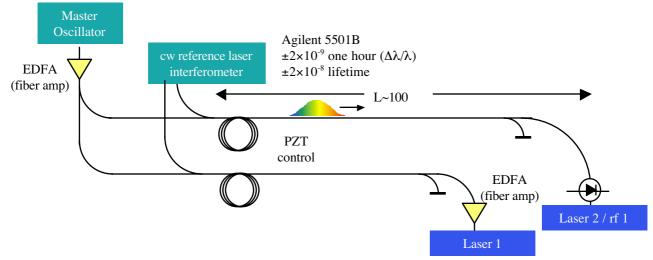
Figure 2. Schematic of fiber distribution network with path length control  $\Delta l = \pm 2 \mu m$ ,  $\Delta t = \pm 7$  fs.
