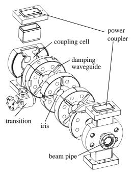
Figure 1: The SICA accelerating structure prototype.
