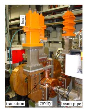
Figure 2: Photography of the accelerating structure installed in the CTF II.
