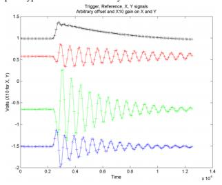
Figure 3: Digitized IF waveforms from the RF cavity BPM's. From top to bottom, the trigger, reference cavity IF and x y IF waveforms are displayed. The time base is in us.
