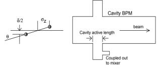
Figure 1: Schematic of the cavity BPM with an incoming 'tilted' beam.
