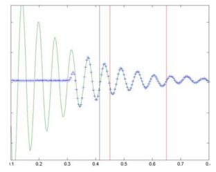
Figure 3: Example waveform with superimposed fit. The fit window is begins about 100 ns following the initial transient.
