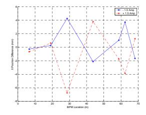
Figure 8: Horizontal trajectory difference when the first horizontal corrector (HC1) change  $\pm$  1.5 A.
