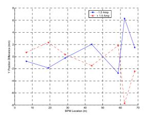
Figure 9: Vertical trajectory difference when the first vertical corrector (VC1) change  $\pm 1.5$  A.
