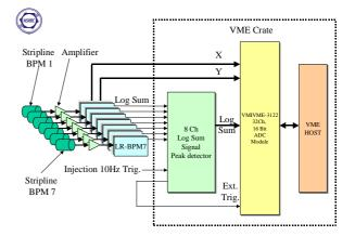
Figure 4: Data Acquisition System for the BTS LR-BPM.
