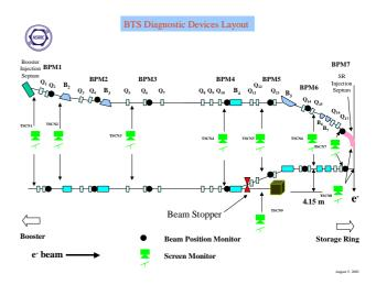
Figure 2: Transport line layout and the BPM installation.
