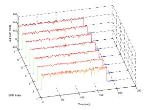
Figure 6: The BTS beam intensity (log sum) distribution as function of time in a routine injection scenario. This figure is shown the log sum output or BTS LR-BPM during injection, the stored beam current of the storage ring is started form 0 mA and accumulate to 200 mA about 170 seconds.
