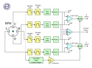
Figure 1: Functional block diagram of the LR-BPM.
