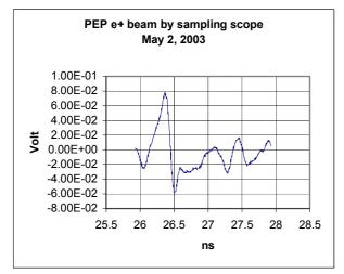
Figure 7: PEP-II e+ Beam Bunch Average Longitudinal Distribution Measured Directly With the TEK 11801 Sampling Scope
