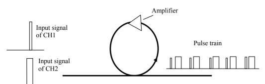
Figure 3: Principle of the Recirculating Loop.
