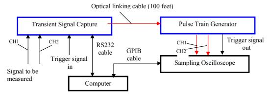
Figure 2: Single-Shot Scope Arrangement. CH, channel.
