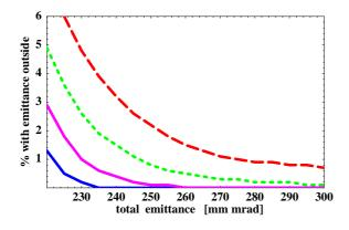
Figure 2: w.p. (6.36,6.22),  $N = 2 \cdot 10^{14}$ : sextupole errors without correction - red (long-dash) line; correction of  $3Q_x = 19$ -green (short-dash); correction of  $3Q_x = 19$ ,  $2Q_y - Q_x = 6$  resonances - pink; no errors - blue (solid).
