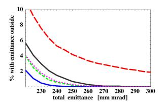
Figure 3: w.p. (6.4,6.3):  $N = 2 \cdot 10^{14}$ , no correction - red (long-dash line); correction of  $3Q_x = 19$  and  $Q_x + 2Q_y = 19$  resonances:  $2 \cdot 10^{14}$ -green (short-dash),  $3 \cdot 10^{14}$ -pink (dotted line),  $4 \cdot 10^{14}$ -black (upper solid line).
