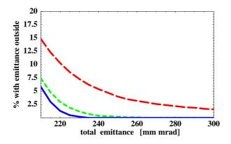
Figure 4: w.p. (6.36,6.22),  $N = 2 \cdot 10^{14}$ : no errors-blue (solid line); octupole and sextupole errors, no correctionred (long-dash line); correction of  $3Q_x = 19$ ,  $2Q_y - Q_x = 6$ , and  $2Q_x + 2Q_y = 25$  resonances-green (short-dash).
