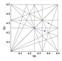
Figure 5: Tune-space with 3rd and 4th order resonances need for correction of w.p. considered.
