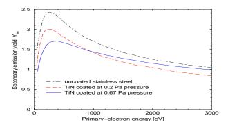
Figure 4: Secondary-electron yield for various coating conditions of the SNS ring chamber measured at CERN. Magnetron (dc) sputtering is used to coat the surfaces with 0.1  $\mu$ m TiN. Surfaces coated at a pressure of 0.67 Pa, which has a lower peak  $Y_{ee}$  but a higher outgassing-rate comparing with those coated at a pressure of 0.2 Pa, are adopted.
