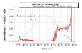
Figure 2: Computer simulation of electron generation in the SNS ring. The beam intensity is  $2 \times 10^{14}$  per bunch. The peak secondary-emission yield (SEY) is assumed to be 2. The peak neutralization level is about 10% within the proton rms beam radius, and about 100% on average within the beam pipe.
