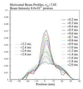
Figure 1: Horizontal beam profiles  $0.2 \sim 2.8$  ms after injection when the horizontal tune was 7.05 and the injection beam intensity was  $8.0 \times 10^{11}$  protons.
