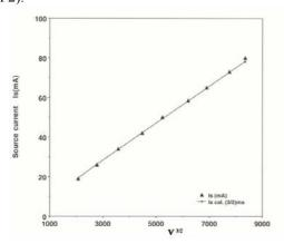
Figure 3: Extracted current from NTX follows Child-Langmuir Law.
