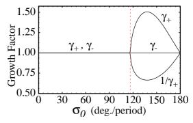
FIG. 2: Phase advances  $(\sigma_{\pm})$  and growth factors  $(\gamma_{\pm})$  for the breathing and quadrupole modes for a thin-lens solenoidal focusing channel and a fully depressed beam. Continuous focusing model predictions for  $\sigma_{\pm}$  are superimposed (dashed curves).
