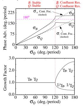
FIG. 3: Phase advance  $(\sigma_Q \text{ and } \sigma_B)$  and growth factors  $(\gamma_Q \text{ and } \gamma_B)$  for the breathing and quadrupole modes for a thinlens FODO quadrupole focusing channel and a fully depressed beam. Continuous focusing model predictions for  $\sigma_\pm$  are superimposed (dashed curves).
