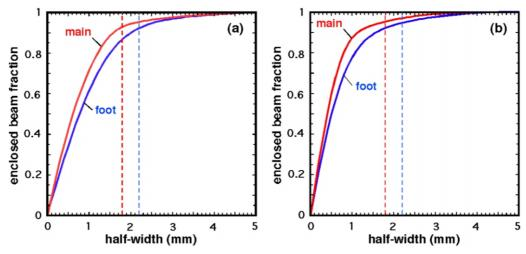
**Figure 2**: Fraction of beam energy deposited within a band of a specified half-width for (a) xenon and (b) bismuth main and foot pulses. Half-widths of the corresponding target annuli are shown as dashed lines.
