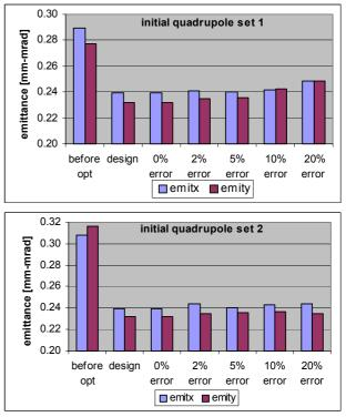
Figure 5: Plots of rms emittances vs. emittance measurement errors. 20% error means that 20% measurement error is included in rms emittance values, which means that  $3\sigma$  of normal error distribution are equal to 20% of the quantity.
