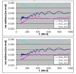
Figure 6: Plots of rms emittance for the cases with 10% (the top plot) and 20% rms beam size measurement uncertainties (the bottom plot). Four wire-scanners are used in series.
