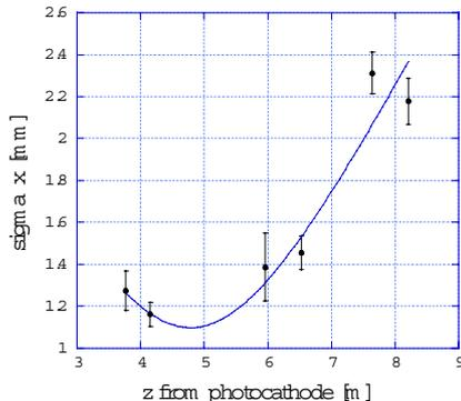
Figure 5: RMS beam envelope in a drift space.
