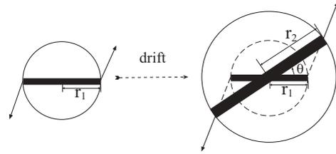
Figure 1: Beam with canonical angular momentum-induced shearing while drifting. The dark narrow rectangular can be a slit inserted into the beam line in order to measure the shearing angle.
