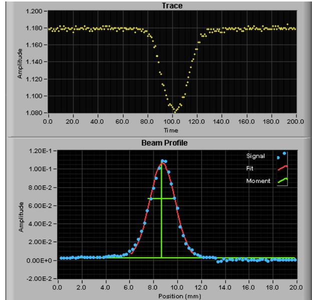
Fig.4. Horizontal beam profile in the SNS MEBT, measured in January 2003. Top: The electron collector signal at the center of the H-minus beam. Bottom: the results of the measurement, with a Gaussian fit plotted out to 2.5  $\sigma$ .
