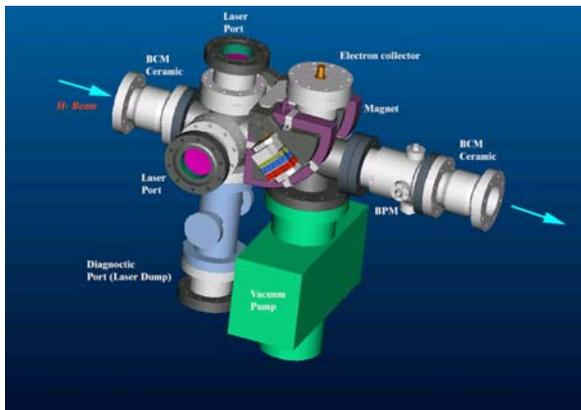
Fig. 2. Stripped electrons are bent into the collector via the dipole magnet (magenta color).
