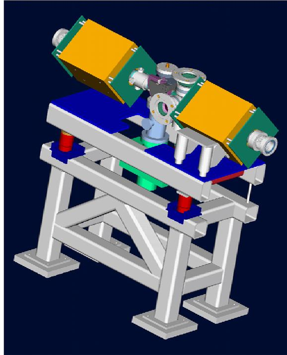
Fig.1. SNS "warm section" is a two quadrupole and diagnostic beam-box located between two super-conducting cavity modules.
