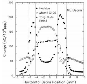
Figure 5: Signals from the Hadron Monitor, 1<sup>st</sup> Muon Monitor, and the target Budal monitor as the beam is scanned horizontally across the NuMI target. The solid (dashed) line represents the inferred outer (inner) edges of the target (collimating baffle).
