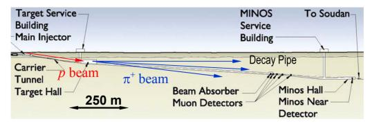
Figure 1: Elevation view of the NuMI beam, indicating primary beam transport, target station, decay volume, beam absorber, muon detectors, and detector hall housing the first MINOS detector.
