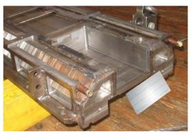
Figure 4: Preparation of the SIS100 test model PDP2 with improved yoke ends (laser-cut slits, reduced stainless steel end plate and minimized brackets).
