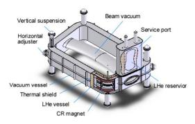
Figure 5: Cryostat structure of a CR dipole.
