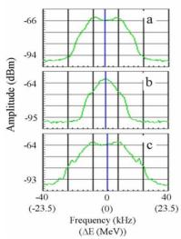
Figure 4. Schottky data for beam in barrier buckets of a)  $T_A$ =2.7 µs, rms  $\sigma_A$ =4.1 MeV,  $\varepsilon_A$ =48 eVs b)  $T_B$ =1.59 µs, rms  $\sigma_B$ =2.2 MeV  $\varepsilon_B$ =14 eVs, (before energy matching and merging,) and c)  $T_{final}$ =3.27 µs, rms  $\sigma$ =4.8 MeV,  $\varepsilon_A$ =68 eVs(after merging using proposed scheme).
