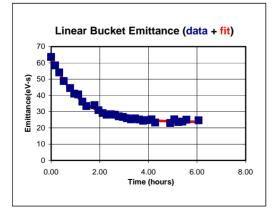
Figure 2: Linear bucket cooling: measured emitttances and model fit.
