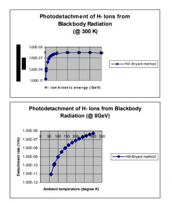
Figure 2: Top – energy dependence of blackbody radiation stripping; bottom – temperature dependence.
